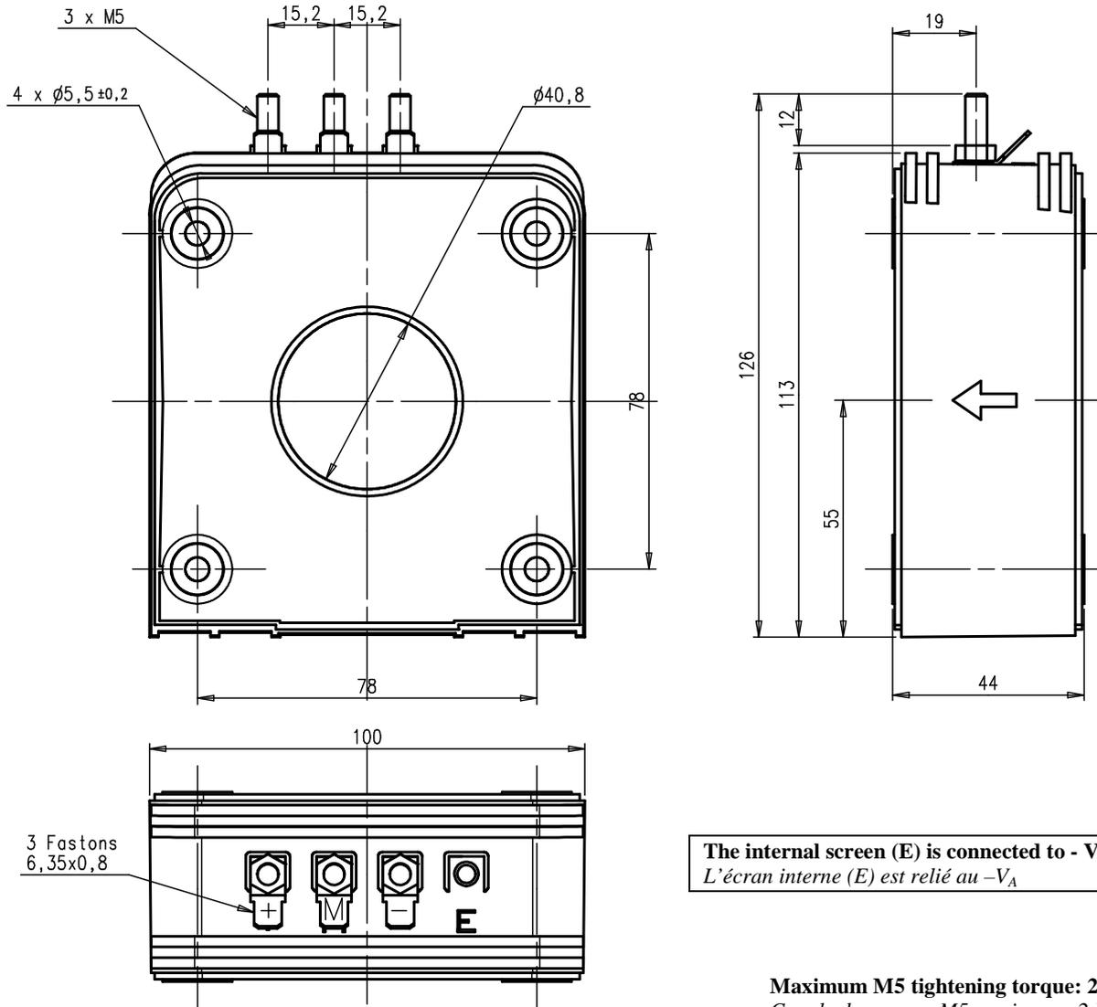
The internal screen (E) is connected to -V<sub>A</sub>
